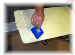
Use the supplied squeegee to quickly spread adhesive down length of Pallet
